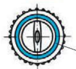
Colored ring marking the spray angle
